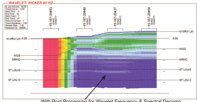
With Post Processing for Wavelet Frequency & Spectral Decomp. Negative Amplitude of Porosity is Clearly Identifiable
